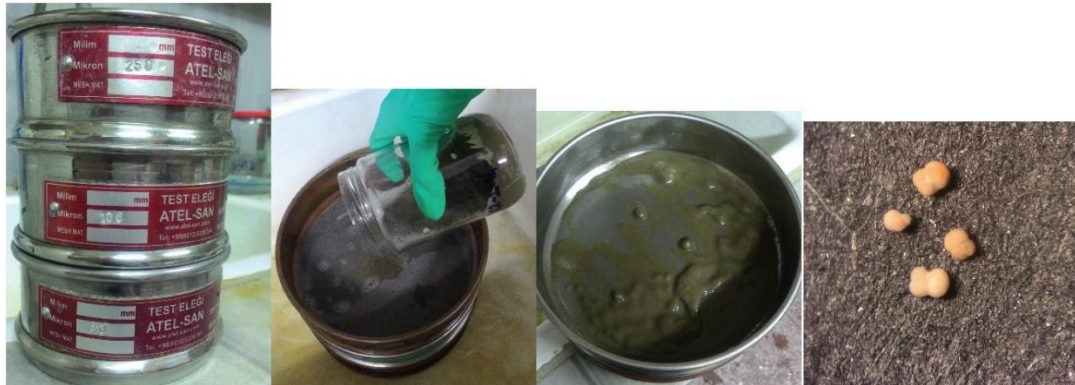
Figure 13: Image of washing samples 250-106-63-micron meters fraction and planktonic foraminifera.
