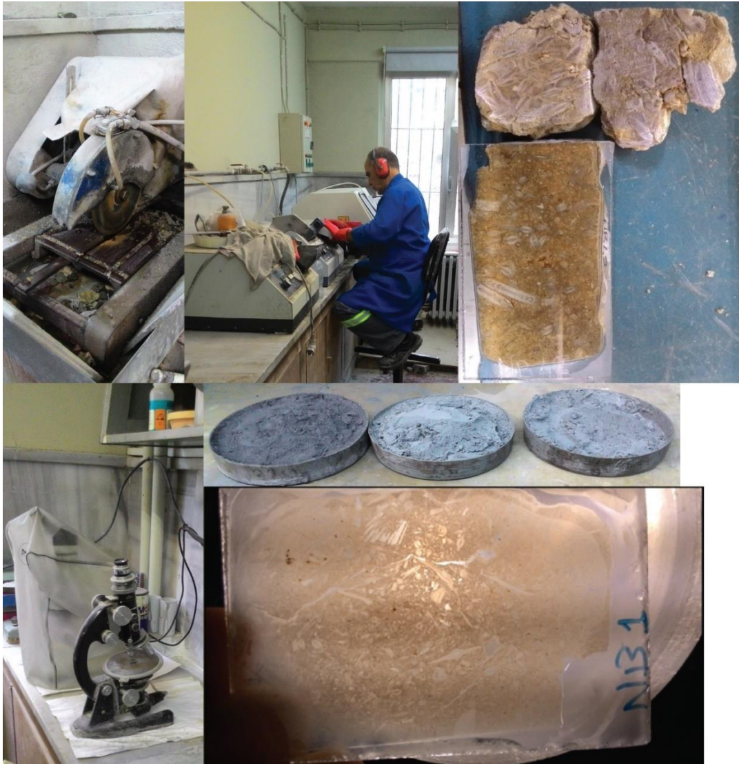
Figure 12: Image of the thin section preparation in the laboratory.
